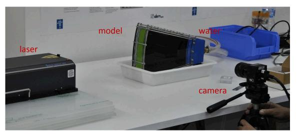
PIV system trial test on a disc sector.
