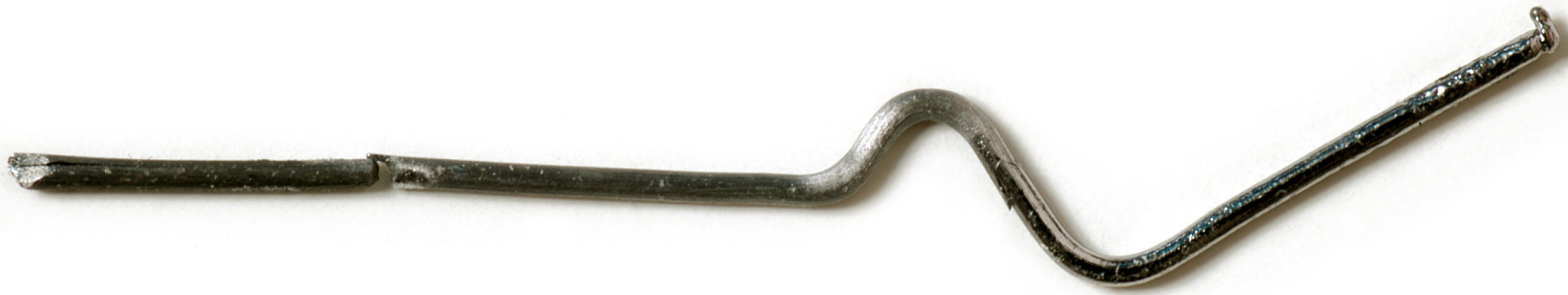
W3 Tungsten Wire, after operating at 4900 A, peak temperature 1800 K, for 3.3 \times 10^6 pulses and then a few pulses at 7200 A at >2000 K.
