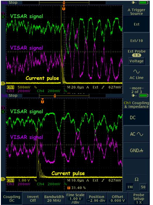
VISAR tests have been performed with 0.3 mm diameter tungsten wire
