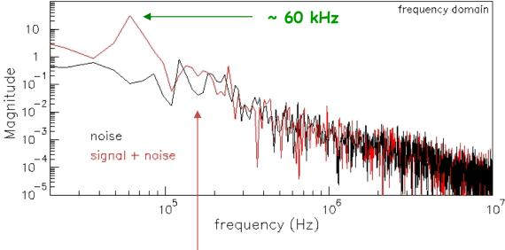
FFT method (MATLAB) has been used - from time to frequency domain -
