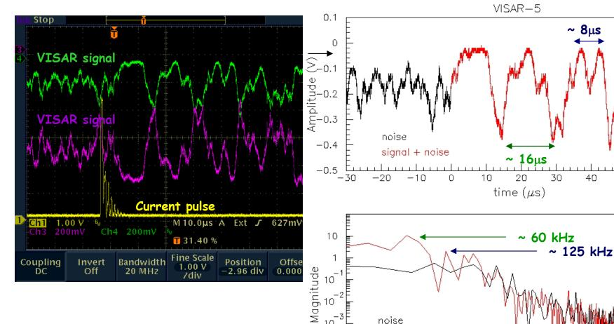
FFT method (MATLAB) has been used - from time to frequency domain -
