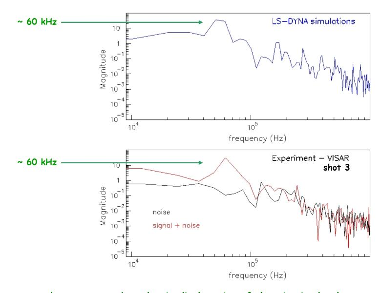
Dominant frequency that corresponds to longitudinal motion of the wire is clearly present in both frequency spectra
