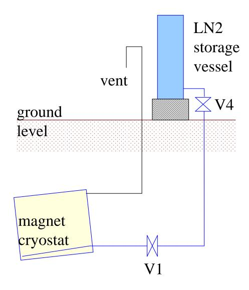
If the cryostat is not emptied before beam pulses, this would reduce the cycle time and give a very simple cryogenic system
