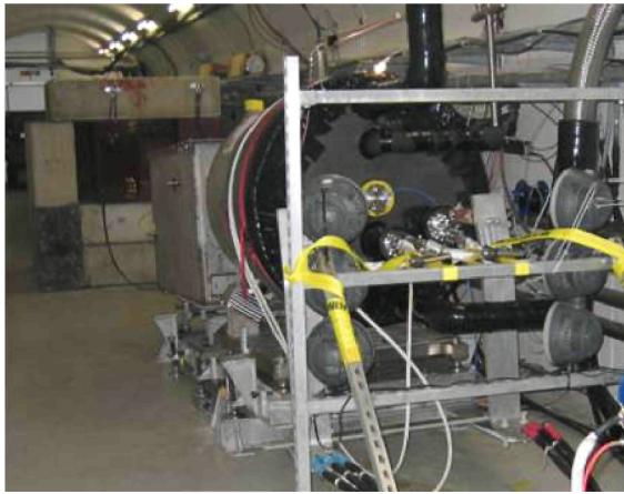
FIGURE 3. The MERIT setup located in the TT2A tunnel of the PS complex at CERN. The picture shows the 15T-solenoid with its bus bars and cryogenic connections. The solenoid bore is occupied by the containment for the mercury jet, which is driven by the piston pump located downstream in the gray box. The direction of the proton beam is into the picture and is stopped by the beam dump seen in the background.
