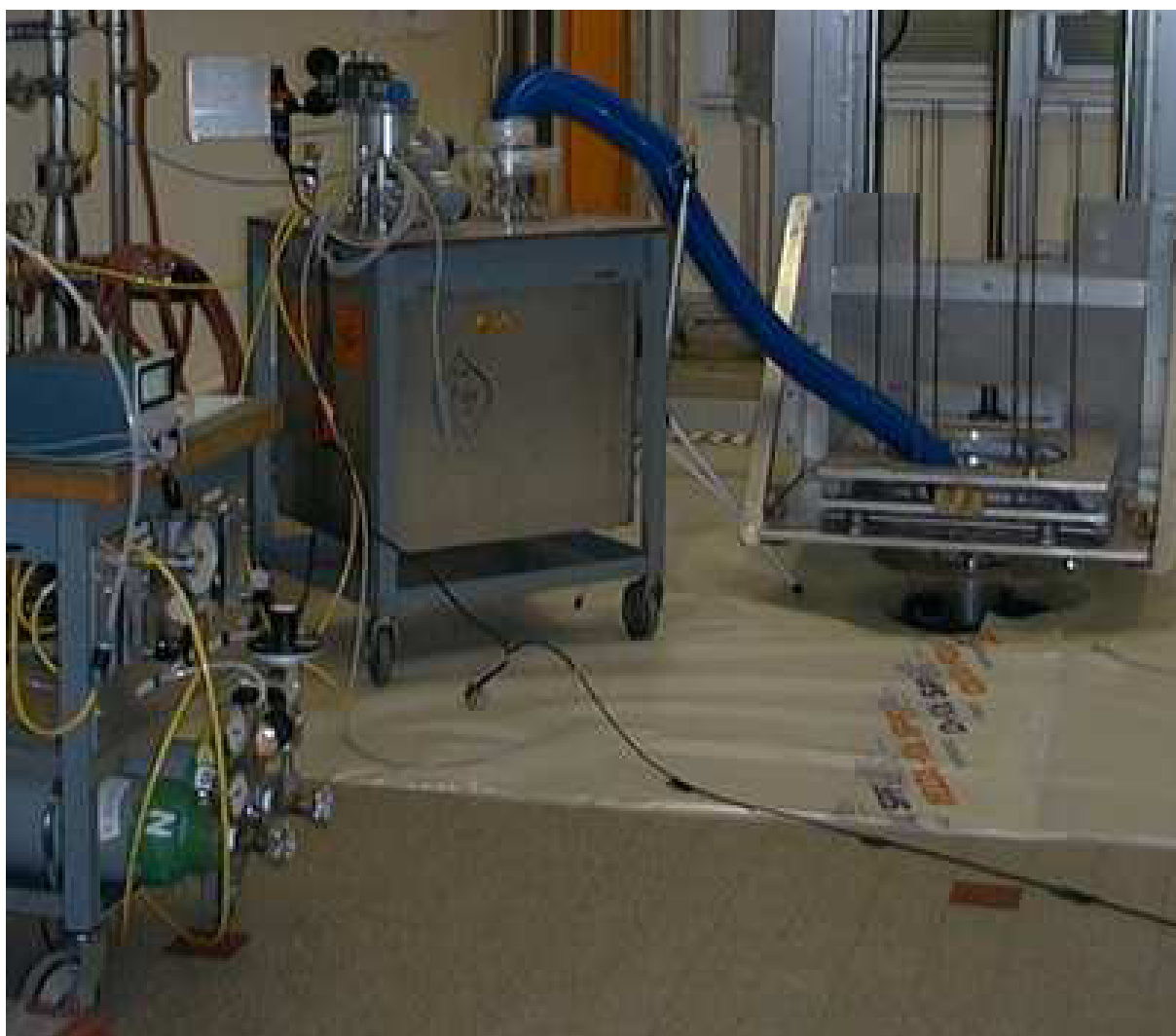
Figure B.1: The experimental setup at GHMFL M9. The vertical bore of the solenoid is lowered in the floor, where the blue hose is pointing to. To the other end the pump device is connected. On the left hand side the gas rack can be seen.
