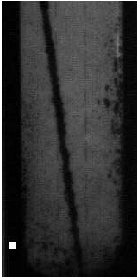
Figure B.4: ... 76 ms after ejected from the nozzle. The splashing of the mercury in backward direction along the steel frame can be seen.
