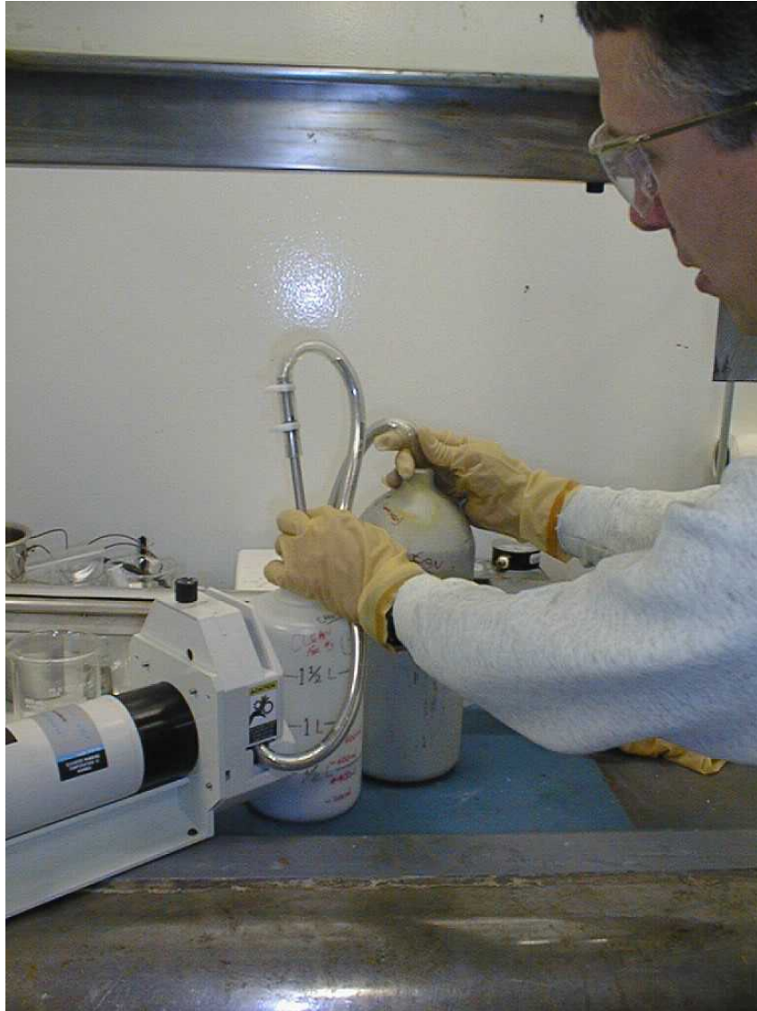
Figure H-2. Pump under operation with mercury in the tube.
