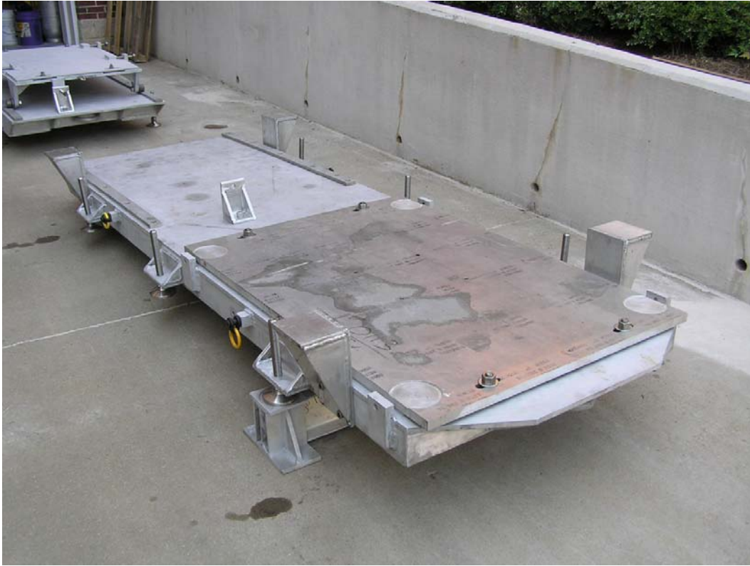
Figure 25. Common baseplate and support beam.
