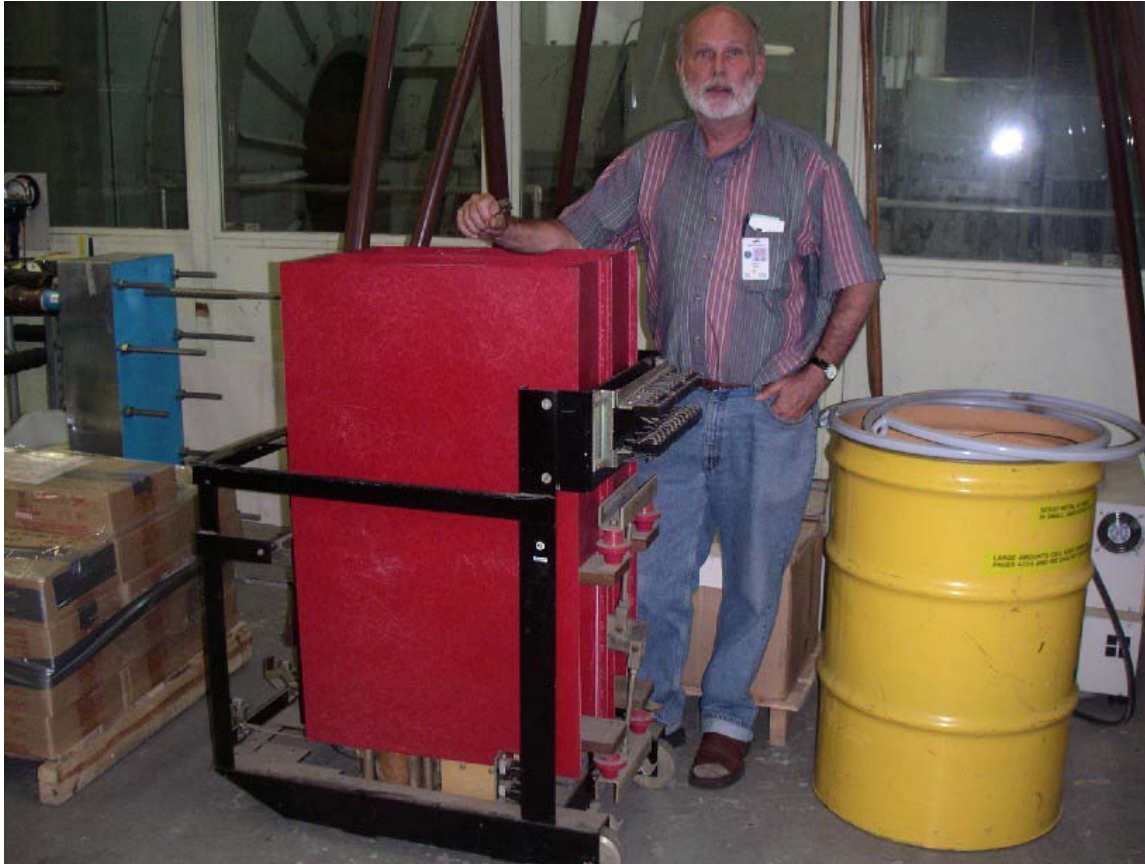
Mechanical Switch capable of 4.4 MW Pulsed System
