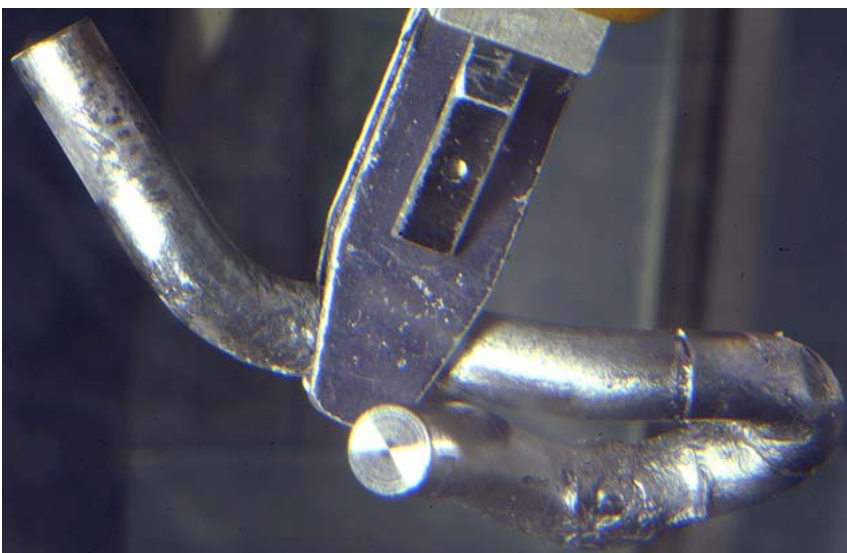
Tantalum rod after one week of ISOLDE running
