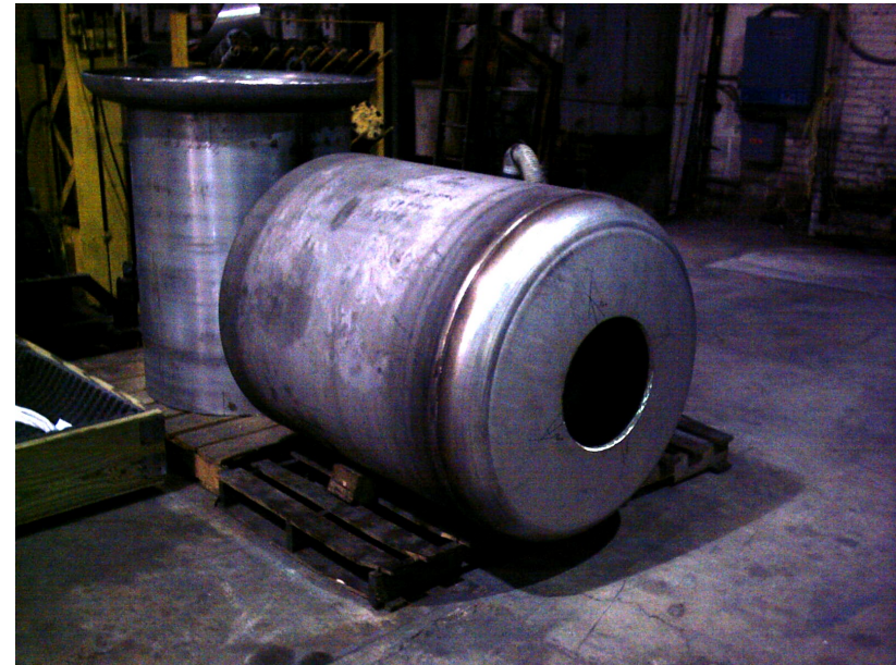
The Cryostat pressure vessel Photo taken April 12, 2005
