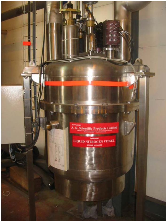
An A.S. Scientific DVB in the Building 180 Test Area
