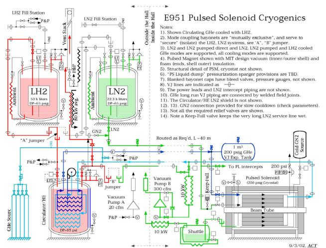
Fig. 3. Piping and Instrument diagram for the proposed cryogenic system to operate a 15-T pulsed, copper solenoid magnet at 30 K.
