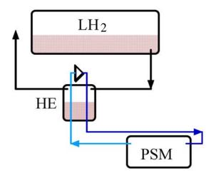
Fig. 2. Concept of the scheme to cool a pulsed solenoid magnet (PSM) by helium gas that is in turn cooled by liquid hydrogen  $(LH_2)$  in a heat exchanger (HE).
