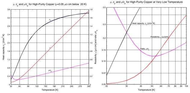
Fig. 1. Left: Electrical resistivity  $\rho$ , heat capacity  $c_p$ , and ratio  $\rho/c_p$  between room temperature and 30 K, for copper with a residual resistivity of 0.05  $\mu\Omega$  cm below ~20 K. Right: Low-temperature electrical resistivity  $\rho$ , heat capacity  $c_p$ , and ratio  $\rho/c_p$  for copper with a residual resistivity of 0.05  $\mu\Omega$  cm below 20 K.
