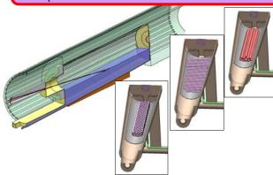
**Above**: Splash mitigation options for the mercury collection pool/beam dump, which will be disrupted by both the proton beam and mercury jet.
