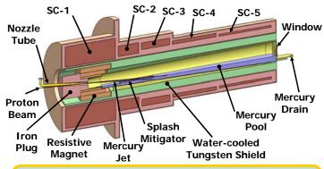
**Concept of a continuous mercury jet target for an intense proton beam.** The jet and beam are tilted by  $\sim 100$  mrad and  $\sim 70$  mrad, respectively, with respect to a 20-T solenoid magnet that conducts low-momentum pions into a decay channel.
