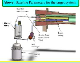
**Above:** A major challenge is incorporation of the proton beam dump Inside the superconducting magnet cryostat. The mercury collection pool can serve as this dump.
