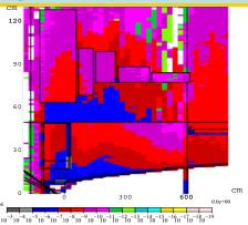
**Above:** Energy deposition in the superconducting magnet and the tungsten-carbide shield inside them. Approximately 2.4 MW must be dissipated in the shield. See also THPEC092.
