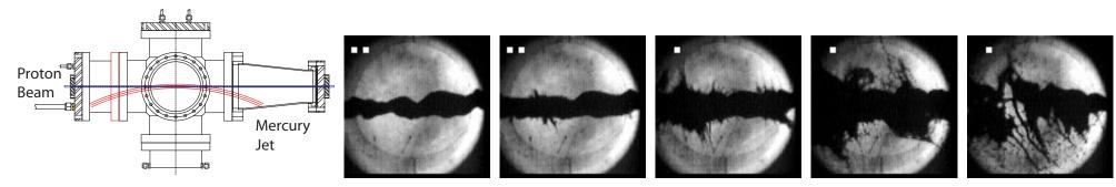
1-cm-diameter Hg jet in 2e12 protons at t = 0, 0.75, 2, 7, 18 ms (BNL E-951, 2001).
