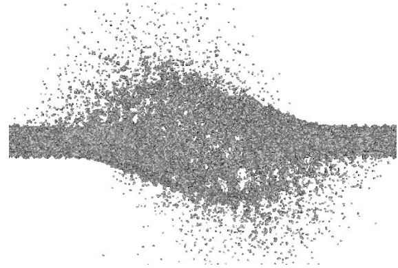
Figure 5: Gallium jet dispersal after proton beam energy deposition.
