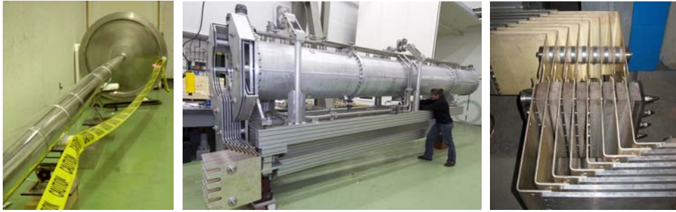
Figures 2a-c: CNGS horn inner conductor, assembled horn and horn-busbar connection.
