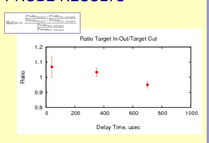
The observed values are consistent with no reduction in particle production for bunches 40 or 350  $\mu s$  after a first set of bunches, and about 5% reduction for bunches delayed by 700  $\mu s$ . This indicates that a mercury jet target, although disrupted by intense proton bunches, would remain fully effective in producing pions during a bunch train of up to 300  $\mu s$  as may be desirable for operation of a **4-MW** proton driver at a Neutrino Factory.
