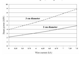
Figure 3: Beam power into a target of 2 and 3 cm diameter versus wire current for the same peak stress (at the initial temperature of 2000 K). Using a proton beam requires that we have 3 bunches at optimum spacing to minimise the stress in the target.
