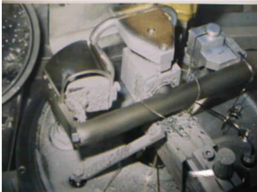
Figure 6: Photograph of an ISOLDE liquid-lead target that ruptured around the upstream window after a few beam pulses [16].
