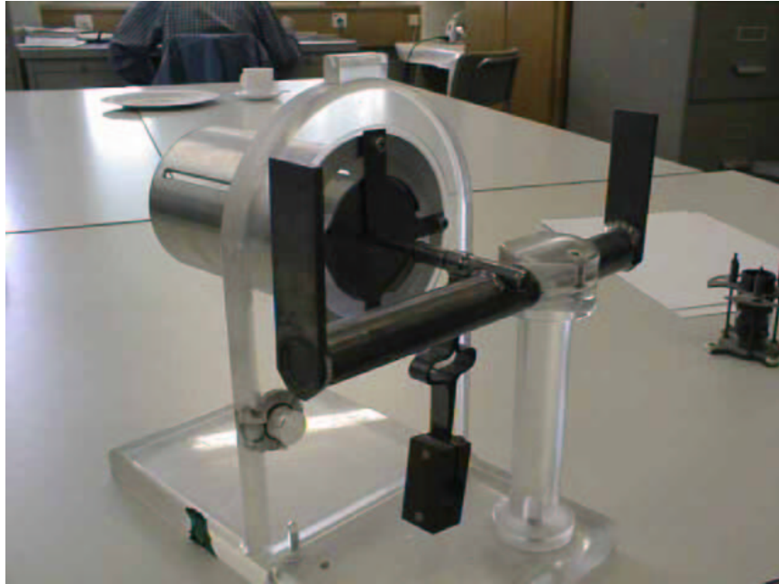
Figure 5: Full-scale model of an ISOLDE target consisting of a 2-cm-diameter, 20-cm-long tantalum cylinder containing molten lead.
