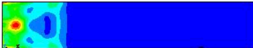
von Mises stress 1.2 micro-secs after pulse
