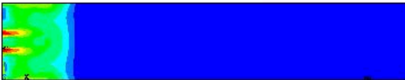
von Mises stress 700 nanosecs after pulse
