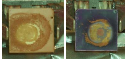
Figure 5. Experimental verification of irradiation temperature using Thermal Sensitive Paint (TSP)
