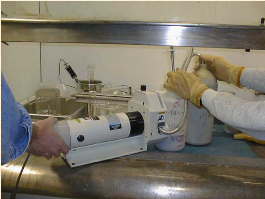
Peristaltic Pump Test
