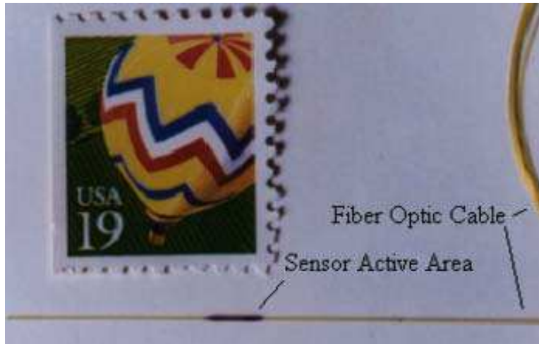
Figure 24: Two-point attachment of the strain sensor.
