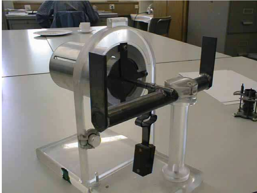
Figure 11: Full-scale model of an ISOLDE target consisting of a 2-cm-diameter, 20-cm-long tantalum cylinder containing molten lead.
