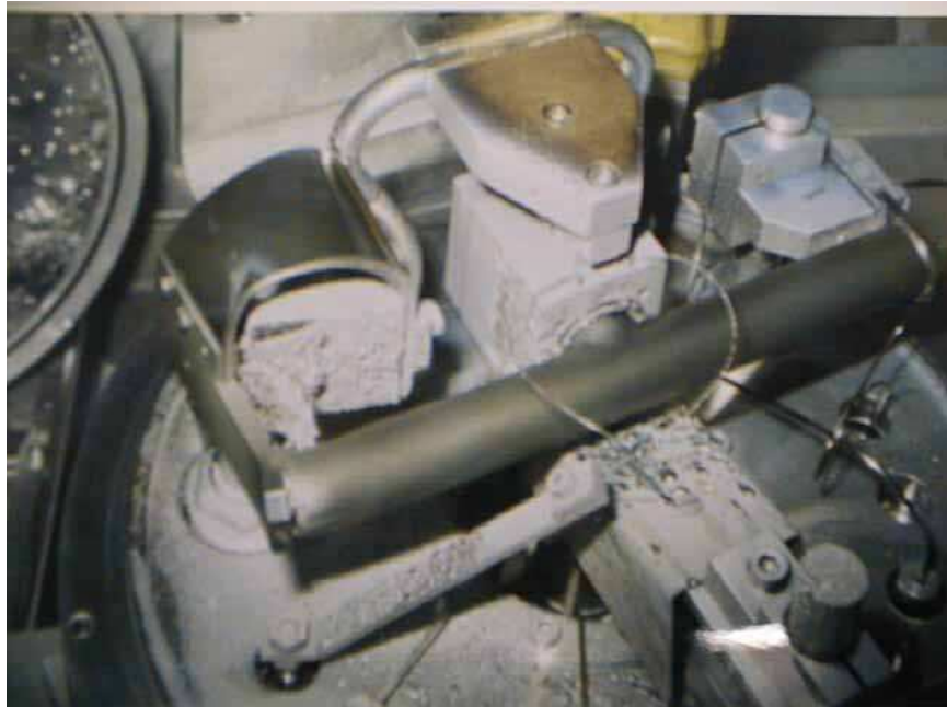
Figure 12: Photograph of an ISOLDE liquid-lead target that ruptured around the upstream window after a few beam pulses [24].
