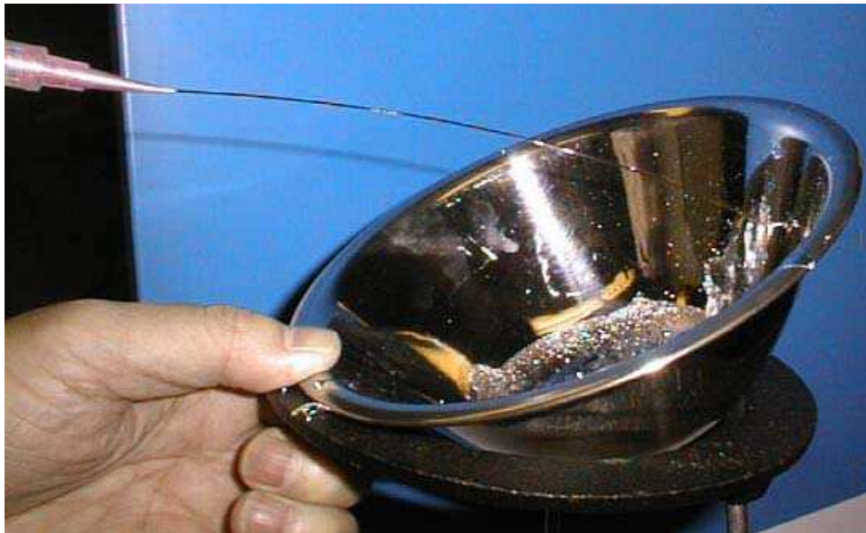
Figure 22: A room-temperature jet of liquid Ga/Sn created by a syringe.
