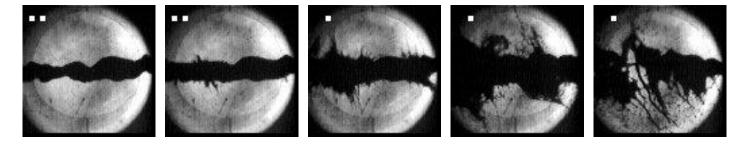
Model:  $v_{\text{dispersal}} = \frac{\Delta r}{\Delta t} = \frac{r\alpha\Delta T}{r/v_{\text{sound}}} = \frac{\alpha U}{C} v_{\text{sound}} \approx 50 \text{ m/s}$ for  $U \approx 100 \text{ J/g}$ .
