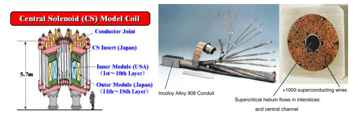
Cable-in-conduit construction similar to ITER central solenoid.
