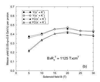
Mercury target radius should be  $\approx 5$  mm, with target axis tilted by  $\approx 100$  mrad to the magnetic axis.
