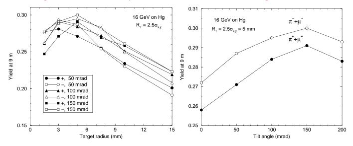
Can capture  $\approx 0.3$  pion per proton with  $50 < P_{\pi} < 400 \text{ MeV}/c$ .
