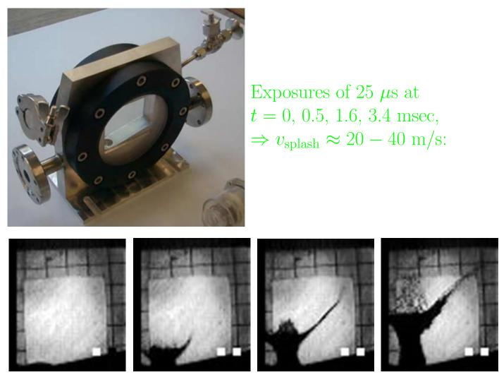
Two pulses of  $\approx 250$  ns give larger dispersal velocity only if separated by less than 3  $\mu$ s.
