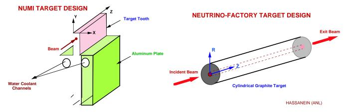
A carbon-carbon composite with near-zero thermal expansion is largely immune to beam-induced pressure waves.
