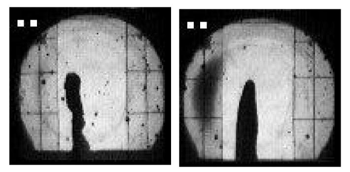
$\Rightarrow$  Damping of surface tension waves (Rayleigh instability).
