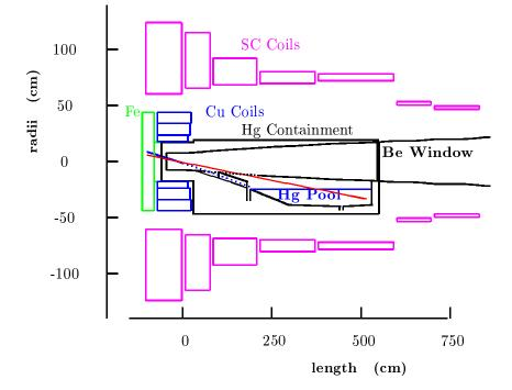
Mercury jet tilted by 100 mrad, proton beam by 67 mrad.
