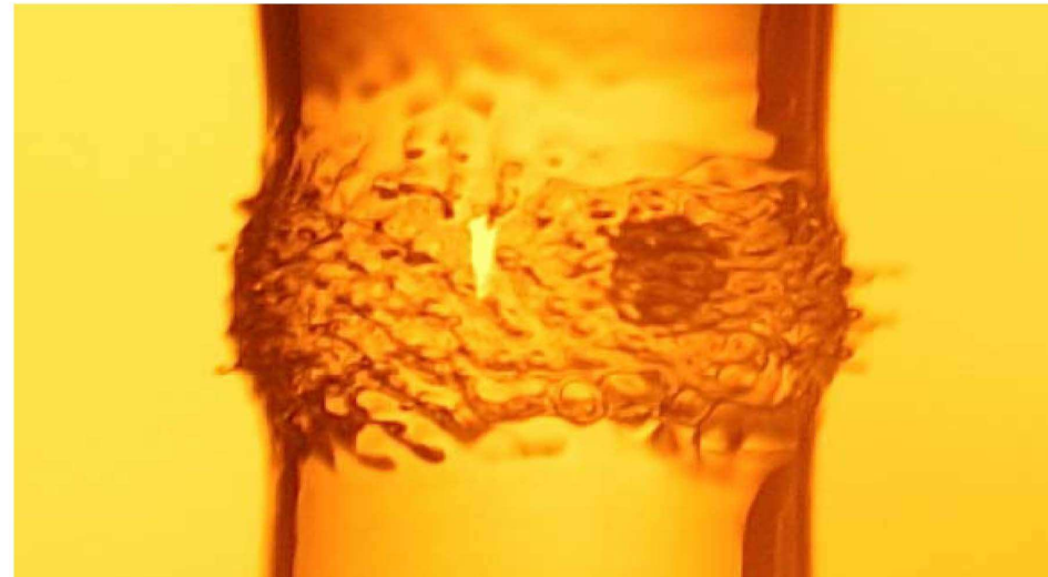
Water jet ripples generated by a 8 mJ Laser cavitation bubble
