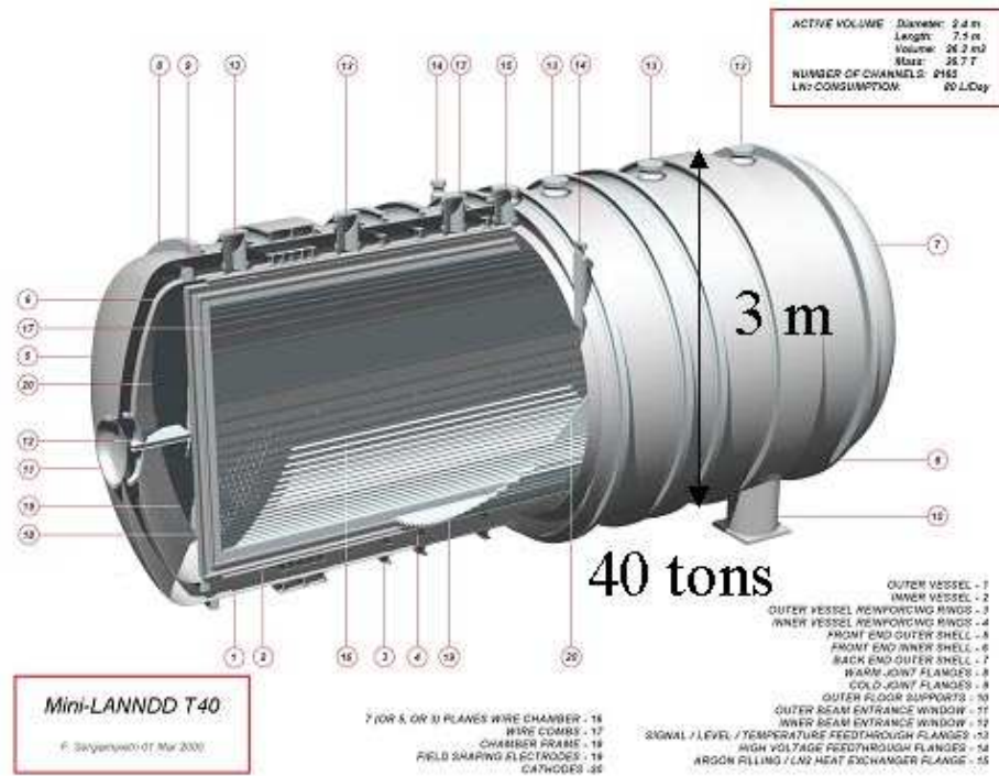
Figure 15: Concept of a 40-ton liquid argon detector for use as an off-axis near detector in the NuMI beam.
