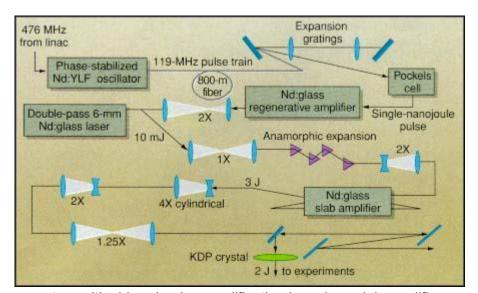
: All-glass laser system with chirped-pulse amplification in a glass-slab amplifier was designed by researchers at the University of Rochester to produce high peak power and high average power for
