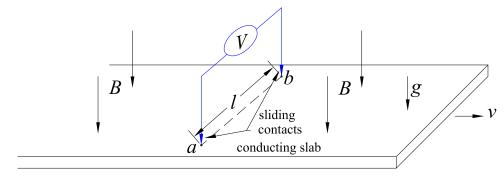
What is the voltage  $(\mathcal{EMF})$  measured by the voltmeter? Consider also the cases where any/all of the slab, voltmeter, and source of the magnetic field move to the right with velocity  $\mathbf{v}$ , supposing that the magnetic field is always uniform in the vicinity of the voltmeter.
