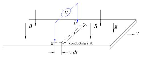
Then, during time dt the magnetic flux through the circuit is  $d\Phi = Blv dt$  in magnitude, and the  $\mathcal{EMF}$  measured by the voltmeter is
