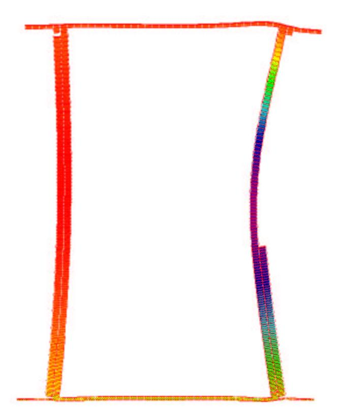
Figure 1: FEA analysis of BABAR endplates coupled by 36-cm-long inner and outer cylinders made of 4- and 8-mm-thick aluminum corresponding to Case 1 in the text.
