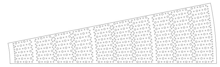
Drilling done at Princeton on CNC mill with Guhring GT100 series parabolic drills.
