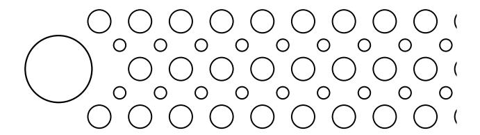
The CMM files are called top179.mea, mid179.mea, bot179.mea, top099.mea and bot099.mea. top, mid and bot refer to the rows of holes, which were drilled from left to right in a given row, one row at a time. 179 and 099 refer to the hole diameters in inches, 4.5 and 2.5 mm, respectively. The files can be found in the anonymous FTP server bbr-boyce.slac.stanford.edu in directory d:\pub-rfb\sands\brenner.
